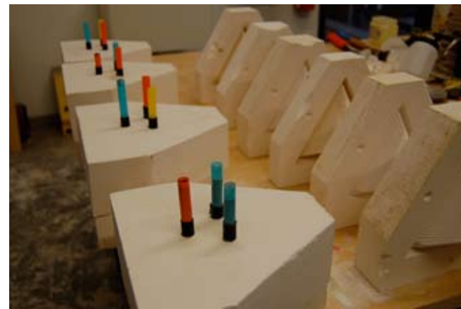
44. Slip casting production line
