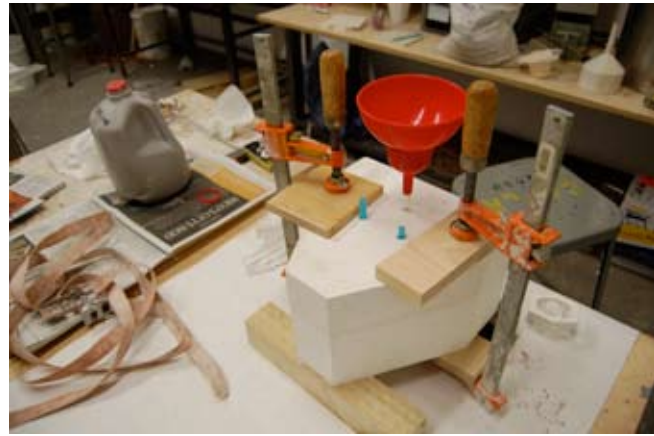
43. Slip casting setup
